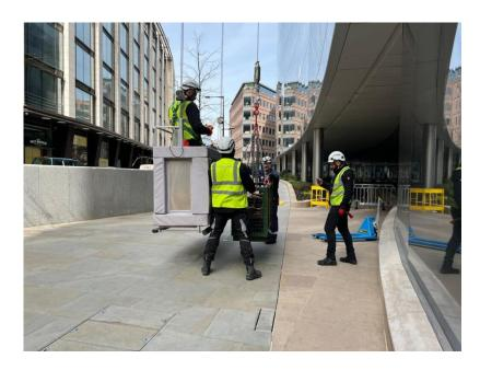
A team of specialist engineers from GIND UK is on site at Plumtree Court in London – the new headquarters of Goldman Sachs – where it is conducting quality and load testing of the building's façade access equipment.
