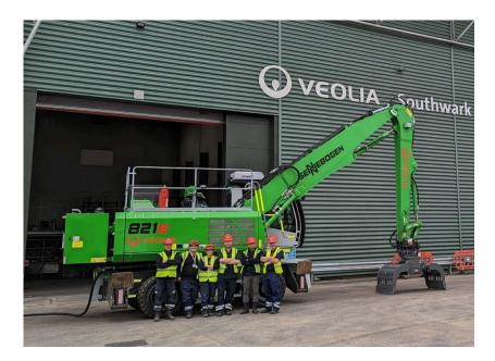
Veolia has introduced their first electric 360 telehandler in the UK. Installed at the company's flagship Integrated Waste Management Facility (IWMF) in Southwark, the telehandler will be used to load the incoming recyclable waste into the bag splitters of the Material Recovery Facility (MRF), which separates the different recyclable materials so they can be sent for reprocessing into new products.
