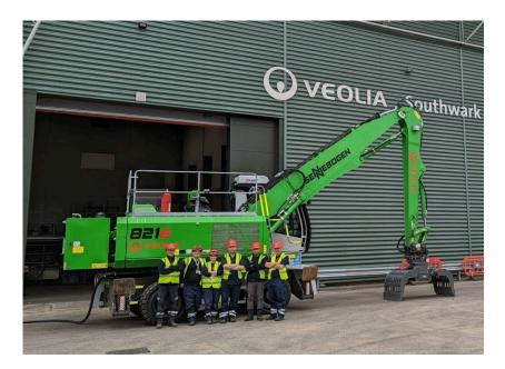
Veolia has introduced their first electric materials handler in the UK. Installed at the company's flagship Integrated Waste Management Facility (IWMF) in Southwark, the materials handler will be used to load the incoming recyclable waste into the bag splitters of the Material Recovery Facility (MRF), which separates the different recyclable materials so they can be sent for reprocessing into new products.
