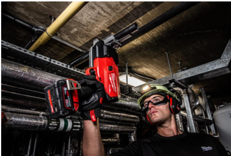
The M18 FUEL™ Steel Pipe Cutter delivers controlled cuts on both installed and new pipes. For installed pipes, the solution's linear blade actuation ensures precise, square cuts, minimising alignment challenges introduced by multi-purpose cutting tools. An integrated positive stop further mitigates the risk of overcuts in tight spaces. For new pipes, the foldable cut fence allows easy, one-handed perpendicular alignment, enabling square cuts without the need for a pipe vise.
