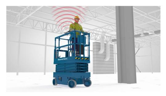
Nationwide Platforms, the UK's leading provider of powered access hire, has launched SkySiren®PCS™ (Pre-Crush Sensor) for Scissors, an industry-first intelligent secondary guarding system designed to significantly reduce the risk of entrapment for scissor lift operators.
