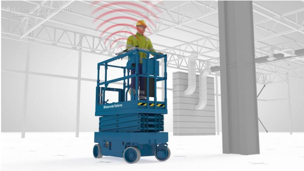
[Nationwide Platforms](#), the UK's leading provider of powered access hire, has launched SkySiren® PCS™ (Pre-Crush Sensor) for Scissors, an industry-first intelligent secondary guarding system designed to significantly reduce the risk of entrapment for scissor lift operators.
