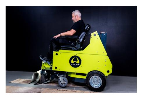
Wolff's first ride-on stripper runs the whole working day powered by <u>Briggs & Stratton's Vanguard</u> lithium-ion commercial battery packs
