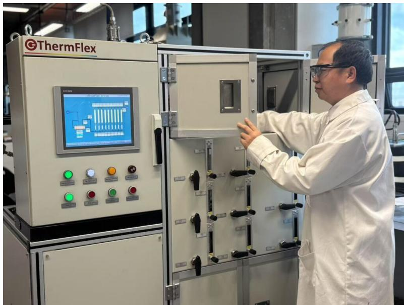
[University of Birmingham](#) researchers have designed a novel energy storage system that could pave the way for decarbonisation of commercial buildings by charging from surplus renewable power that would otherwise be wasted, and delivering heat or cooling when required.
